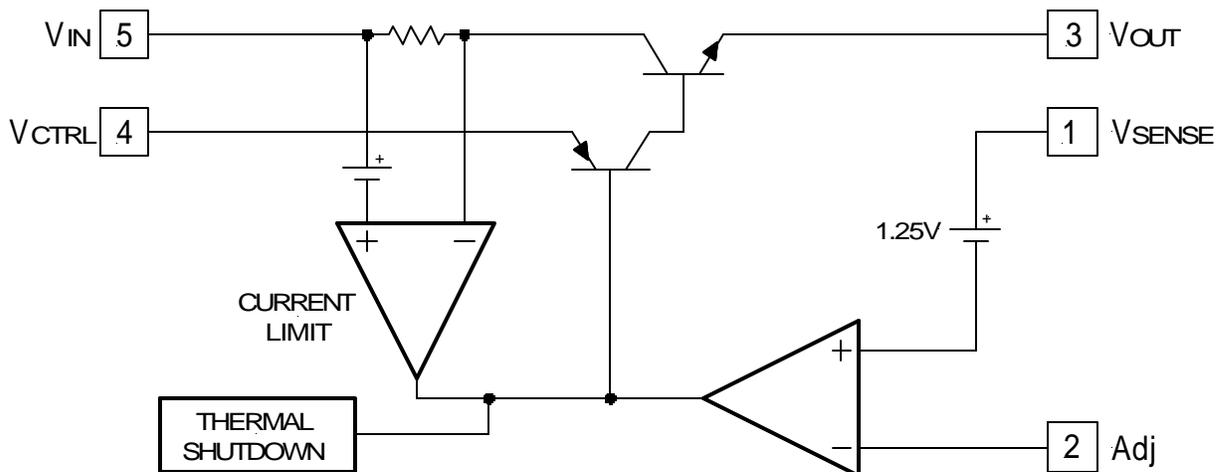
Figure 2 - Simplified block diagram of the APU1160.
