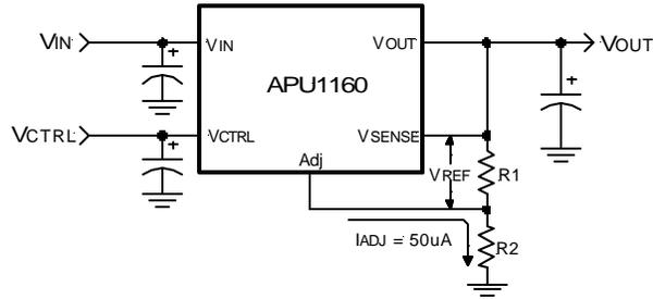
Figure 3 - Typical application of the APU1160 for programming the output voltage.
